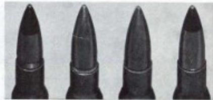
No. 11c. Case Mouth not Crimped in Cannelure
