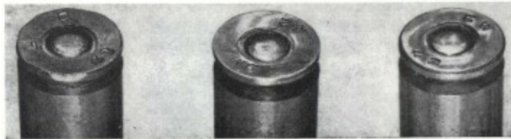
No. 13d. No Chamfer on Head (rim) (Twice normal size, Inclined view)
