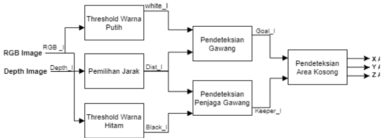
Gambar 3.7 Block Diagram proses vision
