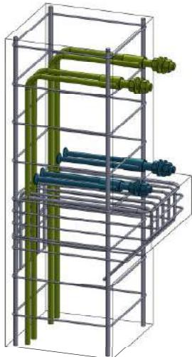
Figure 3. COPRA Anchoring Couplers in a double-sided beam-to-column connection.
