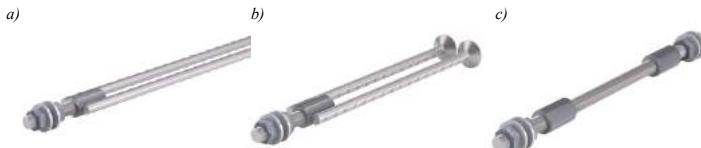
The COPRA P Anchoring Coupler transfers tensile forces by splicing anchor bars to the overlapping main reinforcement of the concrete member. COPRA Anchoring Coupler with straight anchor bars (Figure 1: a) is intended for use in structures with sufficient depth. Alternatively, the anchor bars may be bent to fit in shallow concrete members (see Figure 2).
