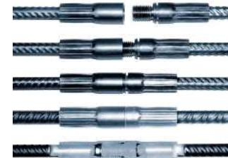
MODIX Rebar Couplers are building products used to create mechanical connections between ribbed reinforcement bars in cast-in-situ and precast concrete structures. MODIX consists of prefabricated female and male muffs with M-threads, which are pressed onto the reinforcement bars. This system provides high production speed with reliable quality. A unique visual inspection system makes the assembly process fast and safe.
