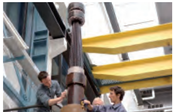
Inspection of a 6-37 anchorage after a leak-tightness test. While being subjected to mechanical and environmental stresses, the anchorage is immersed in a dye solution with a pressure head of 3m.
