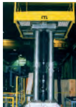
Fatigue test through 2 million cycles
