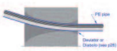
PE pipe through bell-mouth deviator, from anchorage to anchorage (most common detail)
