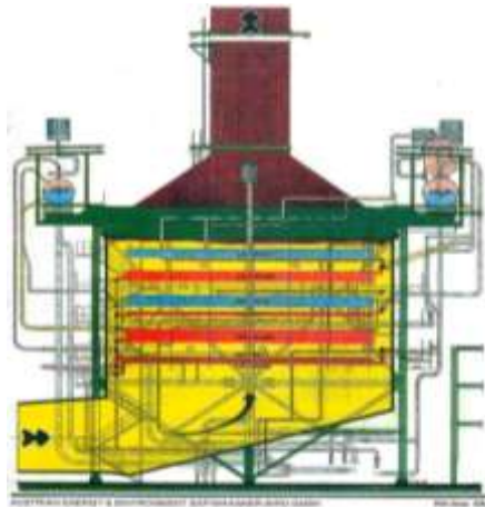
Gambar 1.1 Horizontal Evaporator pada Heat Recovery Steam Generator
