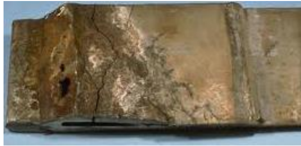
Gambar 2.8 Stress Corrosion (Sumber : metallurgyfordummies.com )
