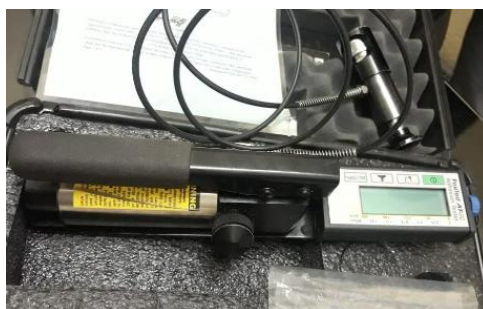
Gambar 3.13 (a) dolly, (b) lem, (c) Portable Adhesion Tester
