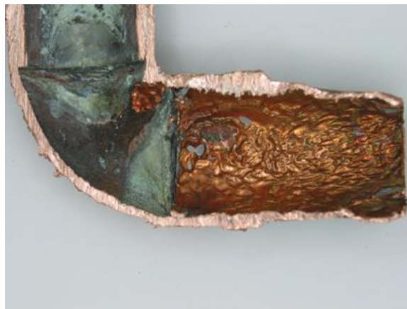
Gambar 2.7 Erosion Corrosion (Sumber : pipingbloging.wordpress.com )
