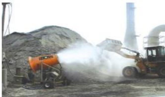
Gambar 4. 20 *Water Fogging Fan*
