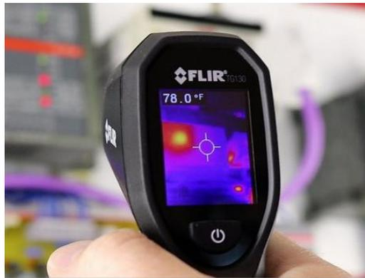
**Gambar 4. 21 Thermal Imaging Spot**
