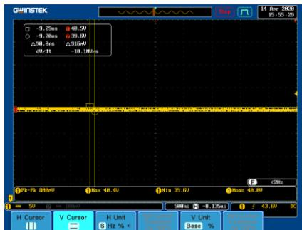
**Gambar 4. 8** Gelombang Tegangan Output Multi-Input DC/DC Konverter
