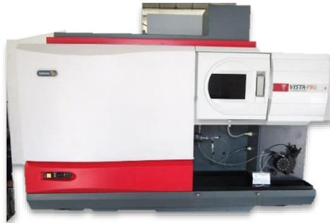
**Gambar 3.5** inductively coupled plasma (ICP-OES, Varian VISTA-PRO CCD
