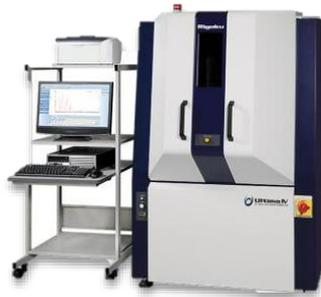
**Gambar 3.4** Alat X-ray diffraction (XRD) Rigaku Rint-2000 . (Ucyildiz, 2017)
