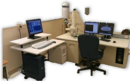
**Gambar 3.2** Alat SEM-XRF tipe JEOL JSM-5600 (Xiao, 2020)
