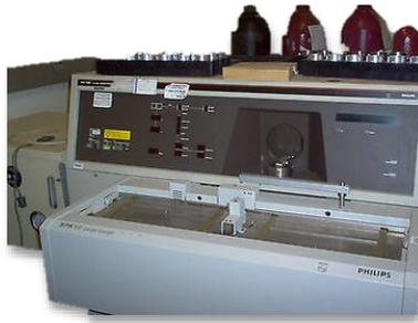
**Gambar 3.3** XRF, Philips PW1480 (Hosseini, 2017)
