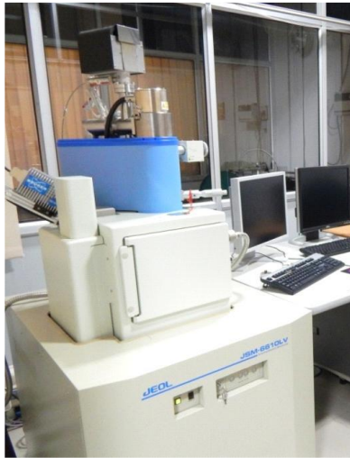
Gambar 3.9 Scanning Electron Microscope (SEM) JEOL JSM-6610LV di Laboratorium EM, G.B. Pant University of Agriculture and Technology, Pattnagar
