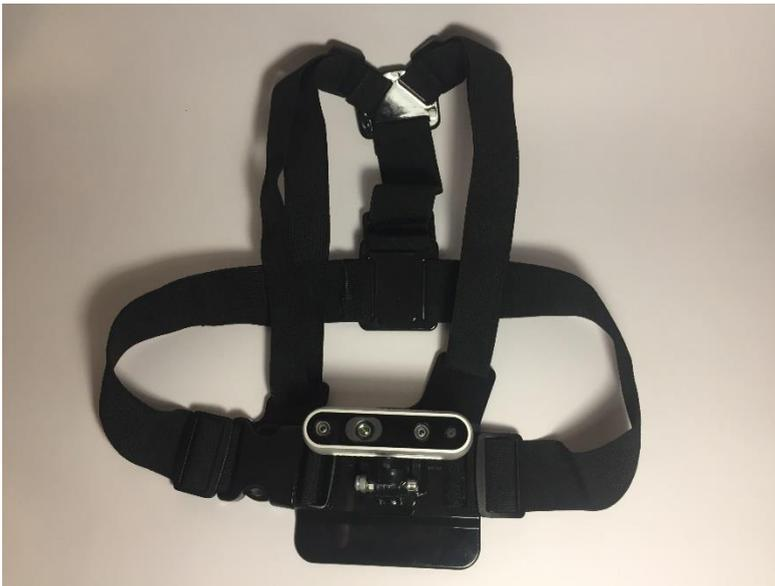
**Gambar 3.4** *Front mounting wearable support*
