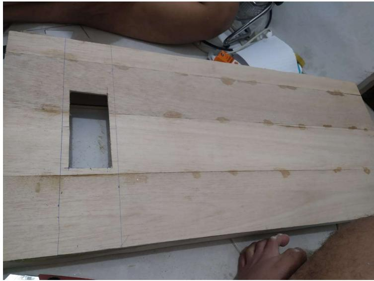
Gambar 4. 62 Kulit *Deck* Prototype Dibolongi
