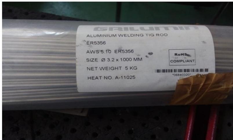
**Gambar 3. 5** Elektroda 5356
