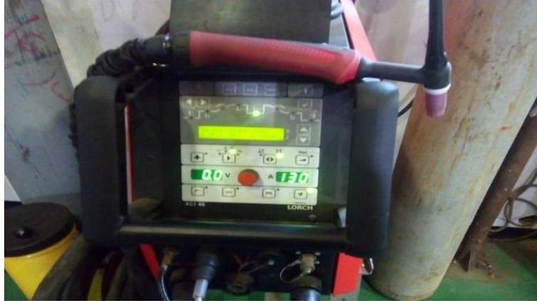
**Gambar 3. 6** Mesin GTAW
