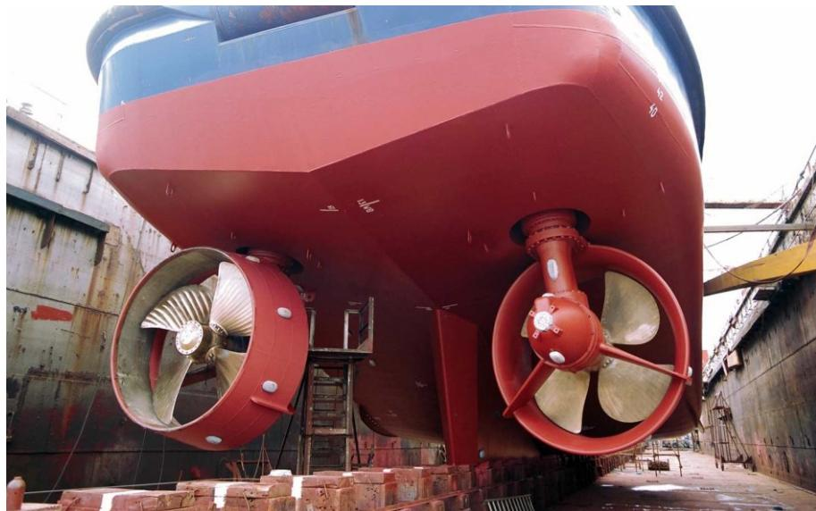
Gambar 2.7 *Tugboat Dengan Tipe Azimuth Thrusters Propulsion with Kort-Nozzle*
