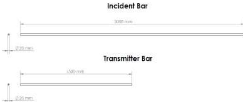
Gambar 3.4 Dimensi *Incident Bar* Dan *Transmitter Bar*
