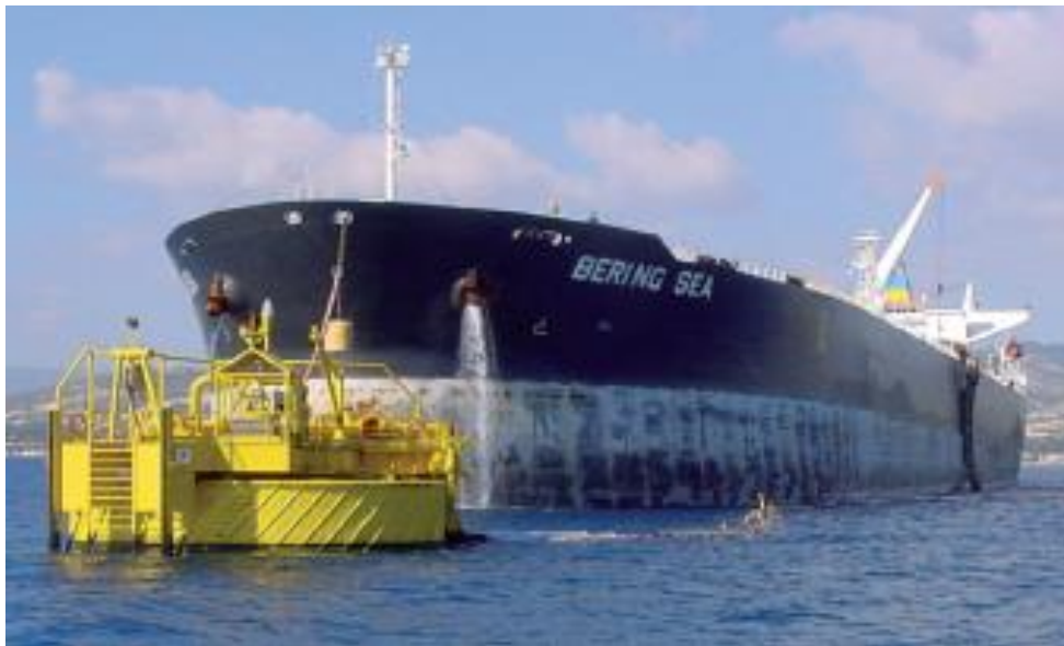
Gambar 1.1 Sistem Tambat Jenis SPM (Sumber : SBM Offshore Catalog, 2012)
