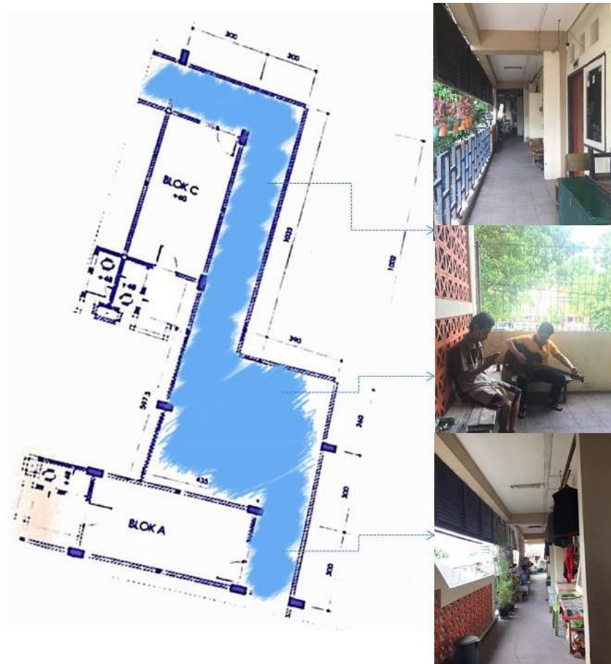
Gambar 4. 23. Koridor Single Loaded Space Design Rusun Urip Sumoharjo
