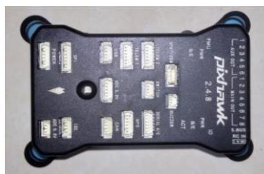
Gambar 2. 1 *Flight controller* pixhawk<sup>1</sup>
