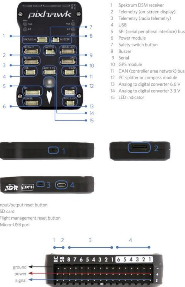
Gambar 2. 2 Pixhawk connector diagram<sup>1</sup>
