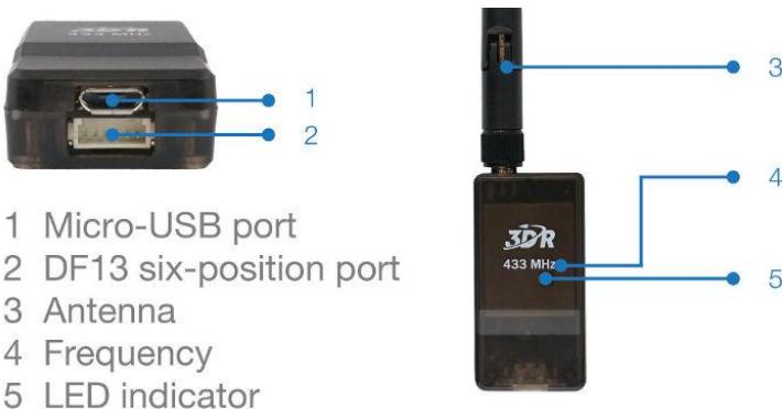
Gambar 2. 11 Telemetry connector diagram
