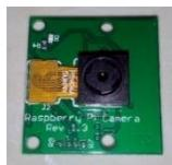
Gambar 2. 16 Raspberry Pi *camera module*
