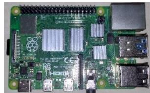
**Gambar 2. 14** Raspberry Pi 4 model B
