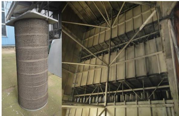
Gambar 2.4 *Inlet Air Filter*
