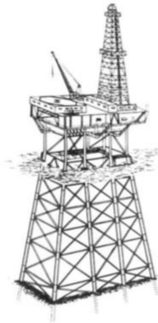
Gambar 2. 1 Gambar struktur jacket platform (Sumber: Chakrabarti, 2005)
