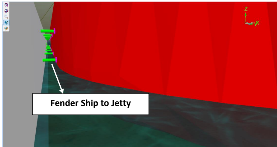
Gambar 4.16 Pemodelan Fender Ship to Jetty
