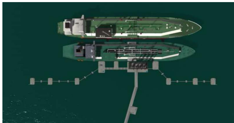
Gambar 2.3 Kondisi side by side Sistem Dolphin Mooring
