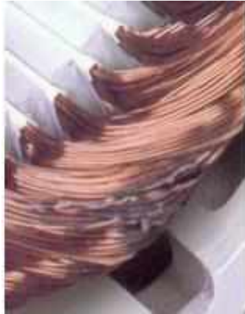
Gambar 2.4 Ilustrasi winding akibat adanya kesalahan stator inter-turn (Yun et al., 2009)
