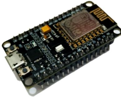
**Gambar 2.7:** NodeMCU ESP8266
