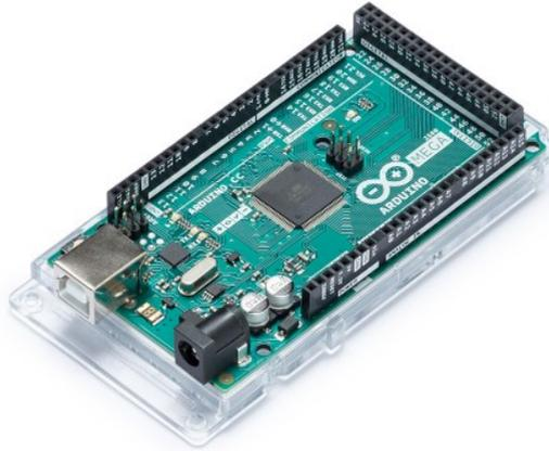
**Gambar 2.6:** Arduino Mega 2560 [4]
