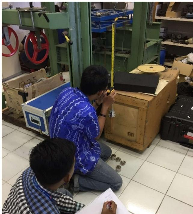
**Gambar 4.10** Proses Kalibrasi Pegas
