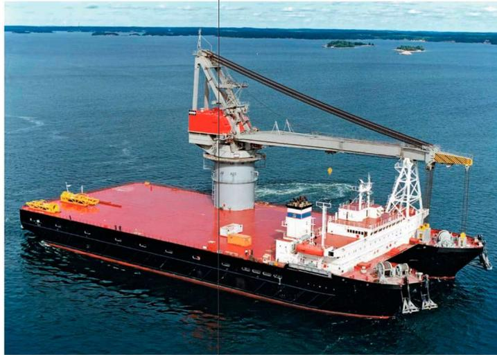
**Gambar 1.1** Struktur *Crane Barge* Tipe Catamaran (Sumber : Titan 2 *Operation at Caspian Sea*)
