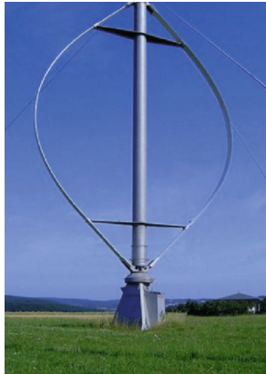
Gambar 2. 2 Vertical Axis Wind Turbine (Md. Rabiul Islam, 2018)
