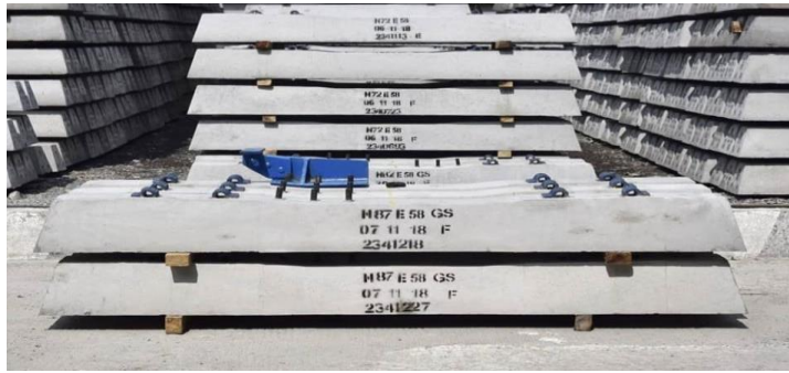
Gambar 4.1 Bantalan jalan rel beton prestressed Sumber: PT WIKA Beton, Pasuruan
