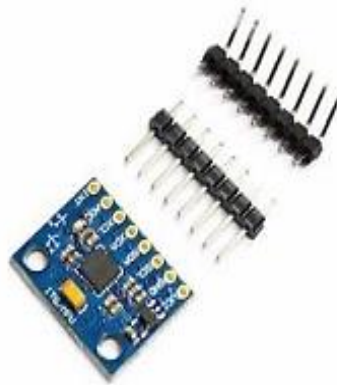
Gambar 3. 6 Modul sensor accelerometer MPU6050 (Gokdemir, 2017)
