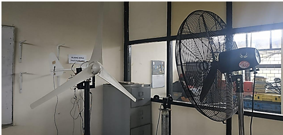
Gambar 3. 2 Set-up monitoring getaran sistem turbin angin
