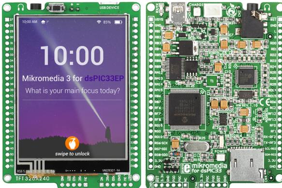
Gambar 2.12: Modul dsPIC33EP [10]
