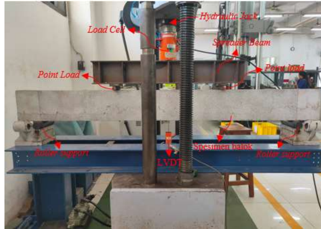
Gambar 3.11. Setup pengujian lentur four point bending
