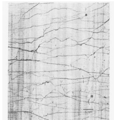
Gambar 2.6. Multiple Cracking in a Spectra ECC (V f = 2%) Uniaxial Tensile Specimen (Li, 1993).
