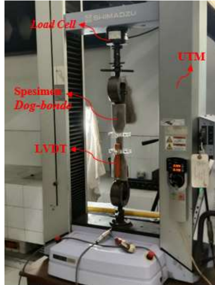
Gambar 3.3. Setup pengujian tarik uniaxial dog-bone .
