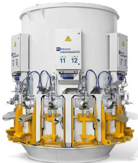
Gambar 1.3 Mesin *Rotary Packing*
