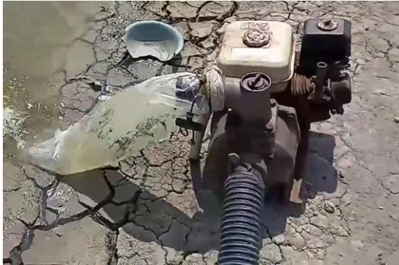
Gambar 4. 6 Pompa Air Sumber : Survey Primer,2020
