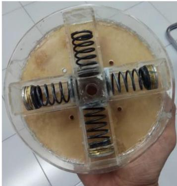
**Gambar 2. 13** *Radial Vibration Damper* (Aufa, 2019)
