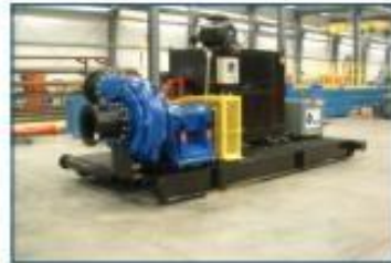
An IMS 1012 Booster Pump on the factory floor ready for shipment.
