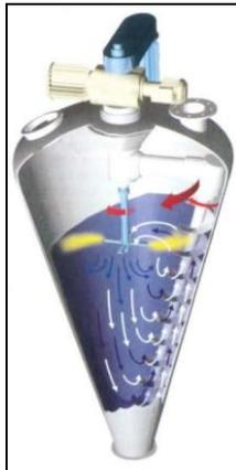
**Gambar 2.3** Ilustrasi mesin *mixing* serbuk (Van Der Wel, 1999)
