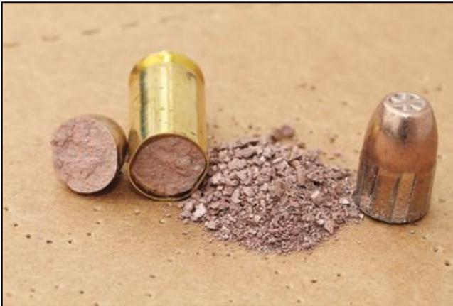
**Gambar 2.2** *Frangible bullet* Cu-Sn10% wt (Rydlo, 2010)
