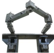
Gambar 2.13 Five-bar Mechanism (Briot, 2015)
