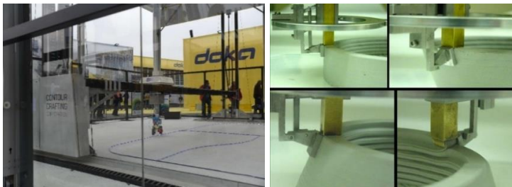
Gambar 1.1. Contour Crafting 3D Construction Printer (Khoshnevis,2004)
