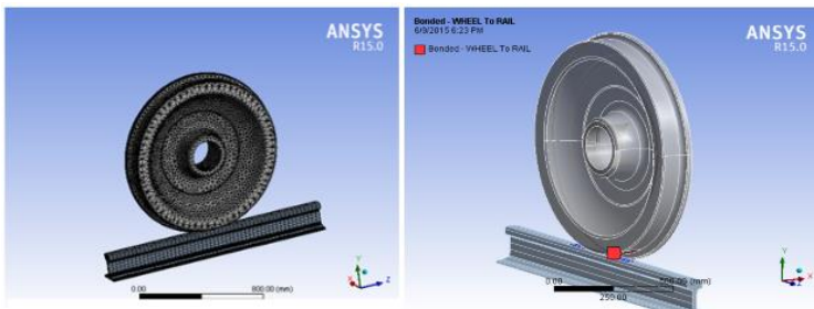
Gambar 2. 12 (a) Permukaan triangular meshing dalam fine quality (b) Bonded contact
