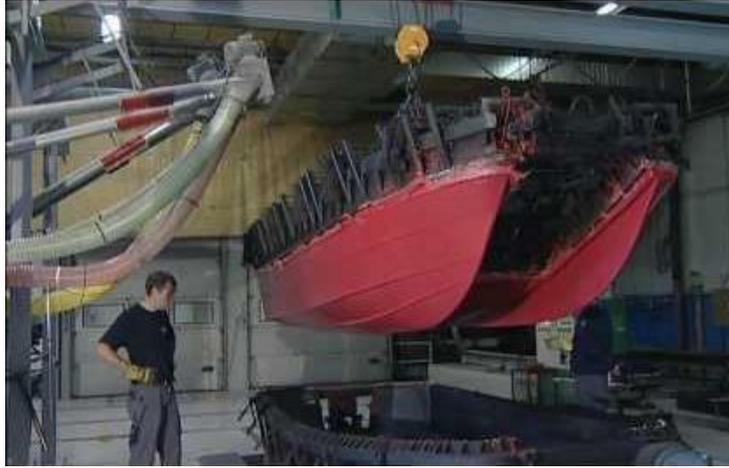
Gambar 2.9 Proses *Rotation Moulding* HDPE
