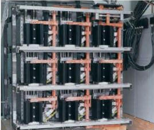
Fig. 12: PEM Fuel Cell modules assembled in a test rack
