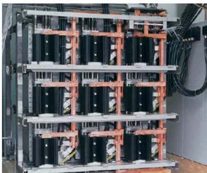
Fig. 12: PEM Fuel Cell modules assembled in a test rack
