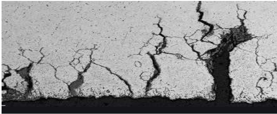
Gambar 2.7 Contoh Stress Corrosion Cracking
