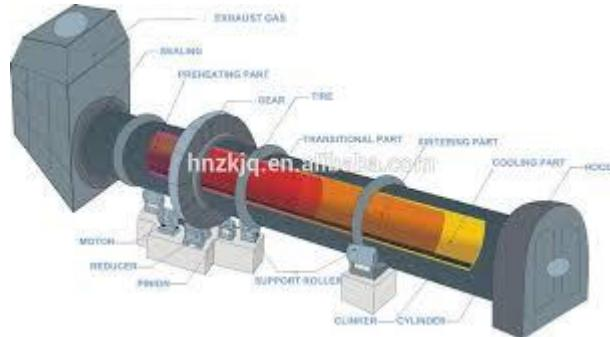
**Fig. 2.2 Kiln** [cementequipment.org]
