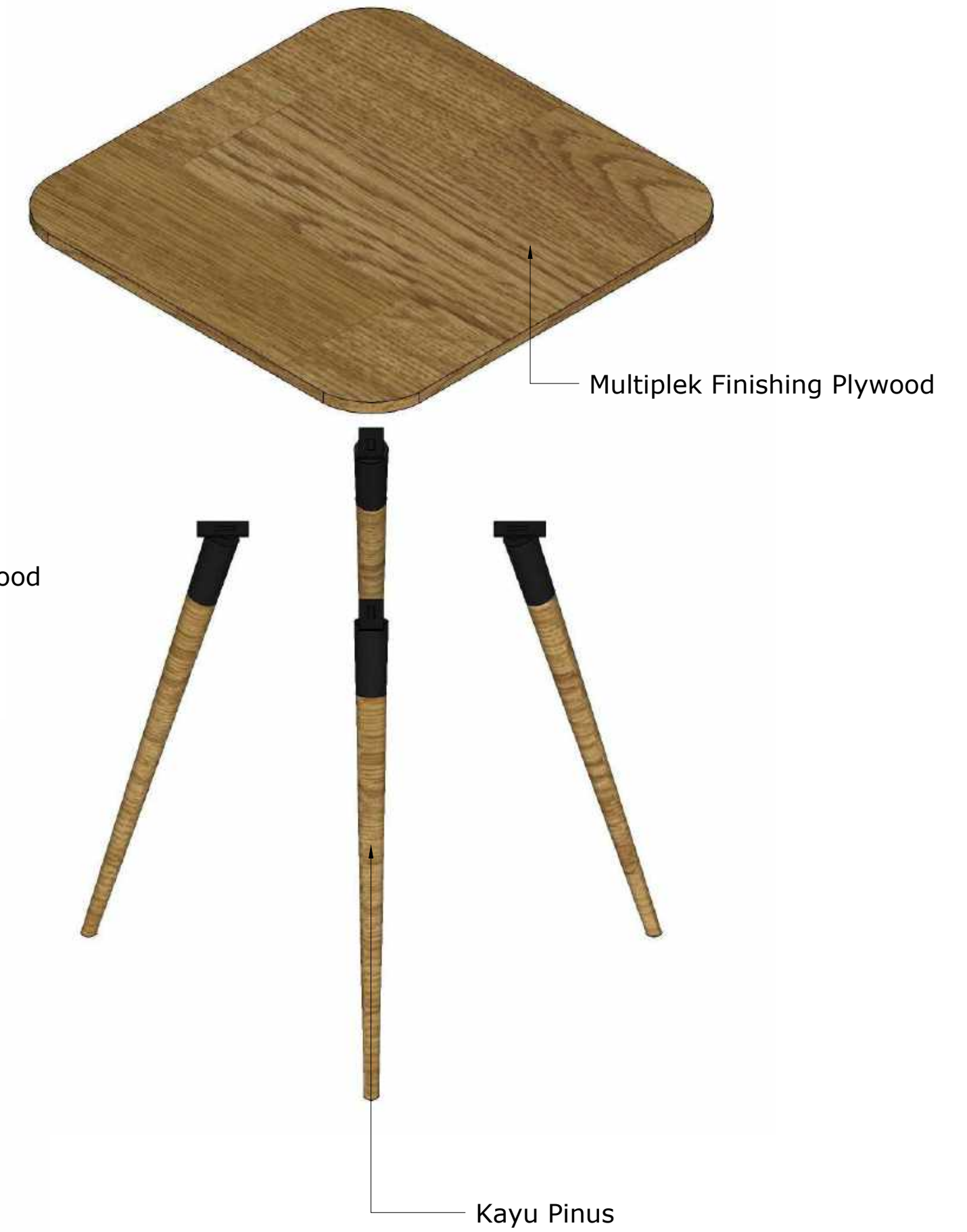
EXPLODED VIEW SKALA 1:7,5
