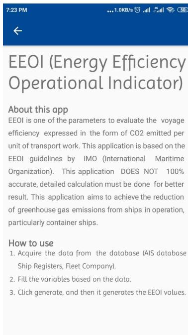
Figure 4.16 About the EEOI Generator Application
