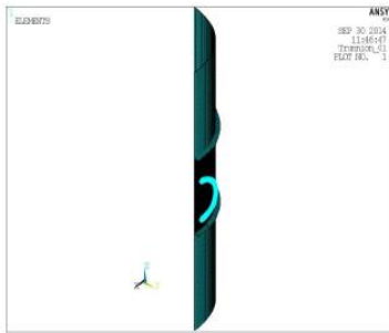
Fig. B.2. Finite Element Model of Trunnion (solid).
