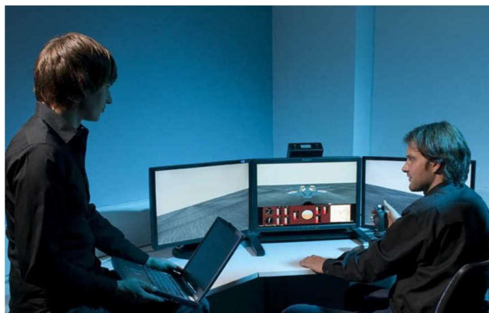
Figure 2.7 WIG simulator with tiled display (Source: Lukas, 2010)
