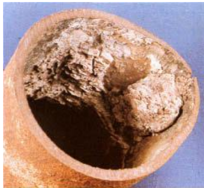
Gambar 2. 4 Endapan Sodium Hydroxide pada Fire-side Wall Tube .(Port, Herro and Robert, 1991)
