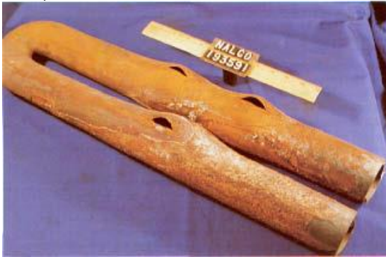
Gambar 2. 12 Bulged dan Ruptured pada Super Heater U-Bend akibat Longterm Over Heating (Port, Herro and Robert, 1991)
