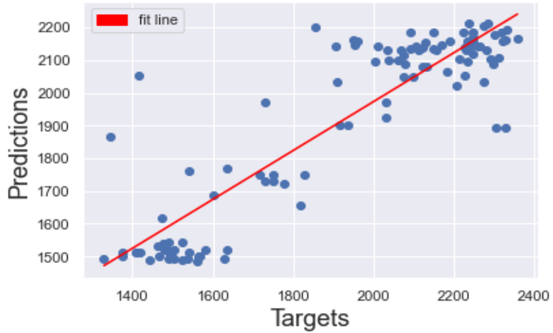
Figure 4. 10 scatter plot of model testing using displacement, engine load, and sea condition as a feature
