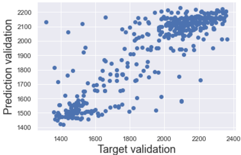
Figure 4. 11 scatter plot of model validation using speed and engine load as a feature
