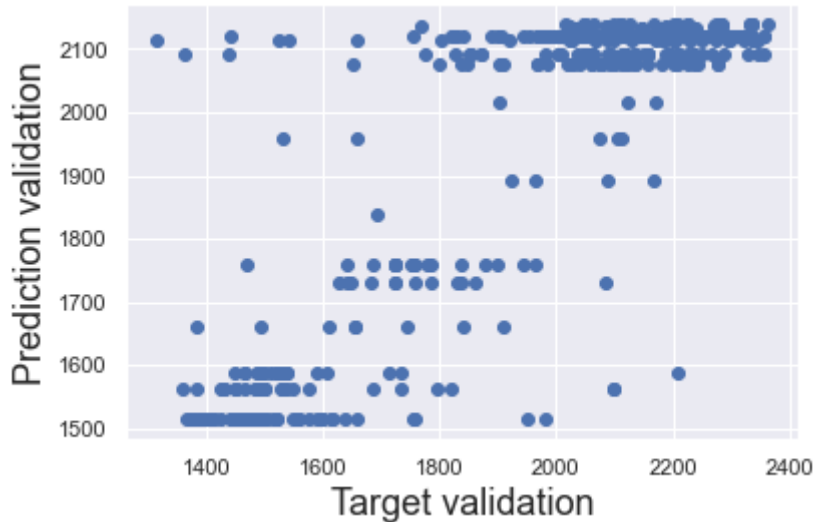
Figure 4. 21 scatter plot of model validation using engine load as a feature
