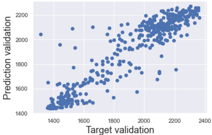
Figure 4. 7 scatter plot of model validation using speed, engine load, and sea condition as a feature
