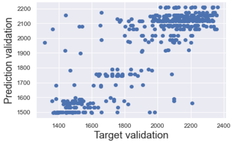
Figure 4. 17 scatter plot of model validation using engine load and sea condition as a feature
