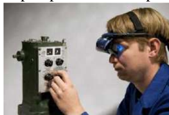
Figure 2.24 Adjustment of a ship engine governor with AR.
