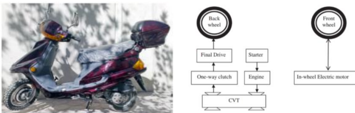
Gambar 2. 1 Hasil manufaktur dan blok diagram hybrid motorcycle powertrain [1]
