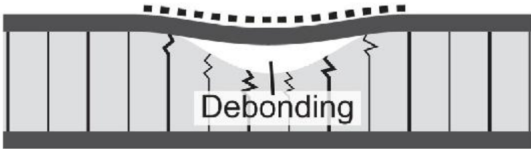
Gambar 2.3 Ilustrasi kerusakan debonding . Sumber: https://www.researchgate.net/
