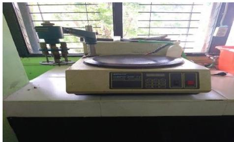
**Gambar 3. 6** Mesin Grinder dan Polisher “ Metcon “
