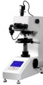
**Gambar 3. 7** Mesin Micro Vickers Hardness
